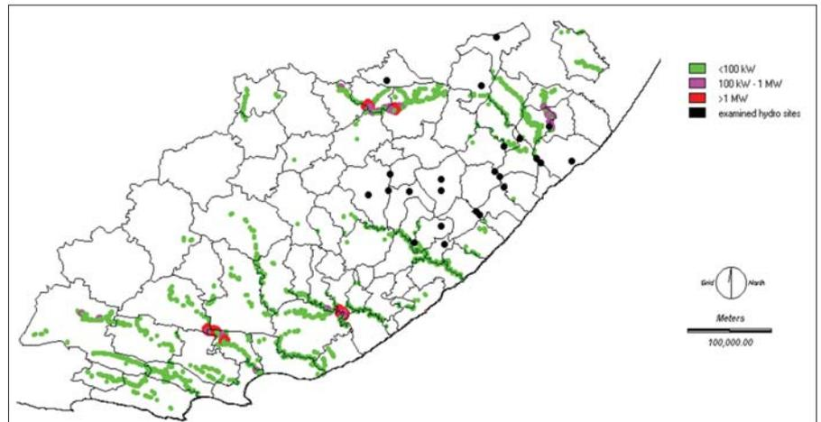
Fig. 10: Small hydropower potential in the Eastern Cape [13].
