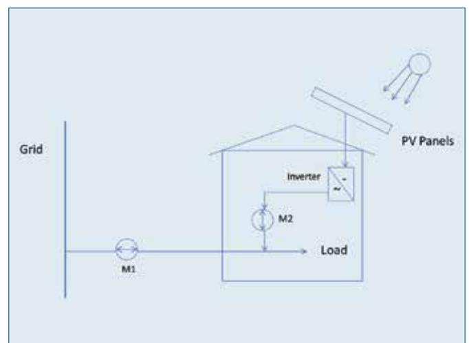
Fig. 3: Possible FIT metering with bi-directional meters.
