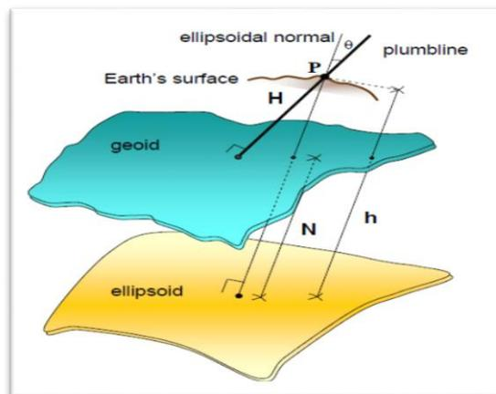
Fig. 1: Relationship between ellipsoidal height ( $h$ ), orthometric height (MSL,  $H$ ) and geoid height ( $N$ )[27].
