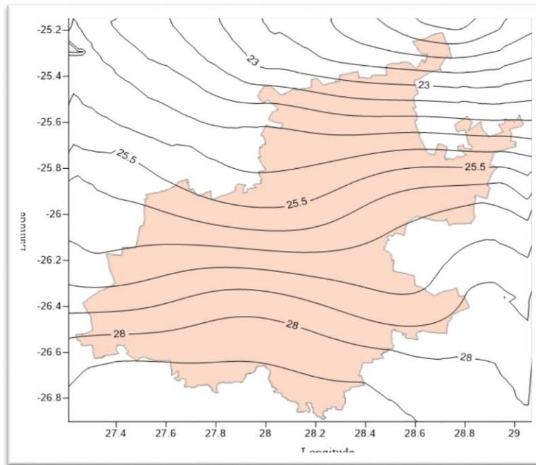
Fig. 2: SiPFFT geoid model at 0,5 m interval contour plot.
