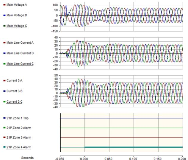
**FIGURE 16: Operation of the modified algorithm for reverse fault**
