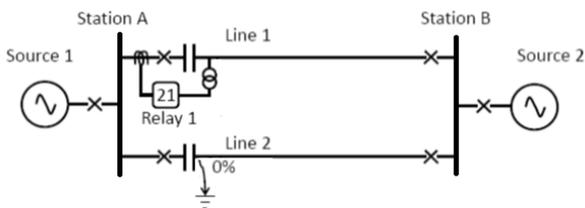
**FIGURE 14: Reverse fault on double circuit transmission line**
