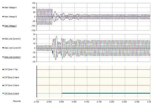
**FIGURE 10: Correct zone operation during reverse faults (modified algorithm)**
