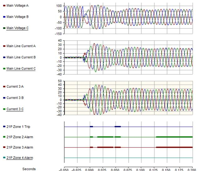
**FIGURE 17: Operation of the non-modified algorithm for reverse fault**
