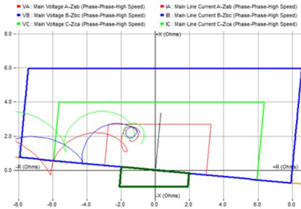
**FIGURE 1: Mis-operation distance relay during voltage inversion.**
