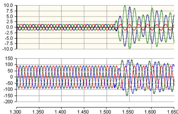
**FIGURE 2: Typical sub-harmonic waveform [11]**
