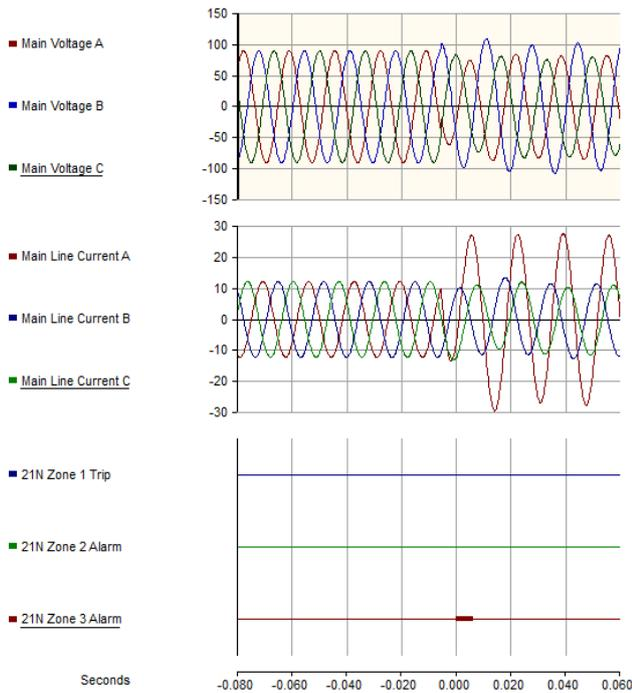
**FIGURE 13: Incorrect operation during forward high impedance fault (non-modified algorithm)**
