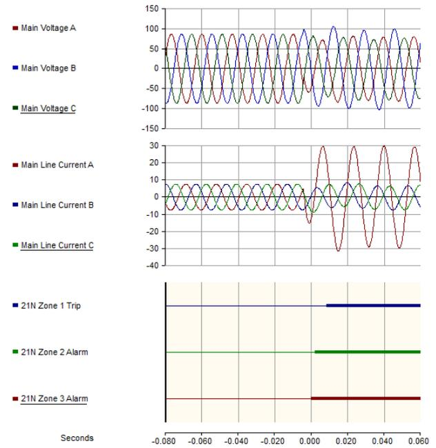
**FIGURE 12: Correct zone-1 operation during forward high impedance fault (modified algorithm)**
