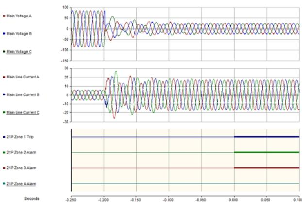
**FIGURE 11: Zones mis-operation during reverse faults (no-modified algorithm)**
