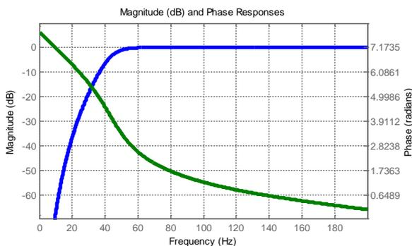
**FIGURE 4: Sub-harmonic removal filter response (50 Hz system) [11]**
