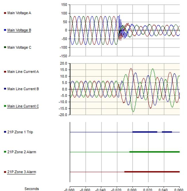
**FIGURE 9: Zone-1 over-reach due to sub-harmonics (no-modified algorithm)**
