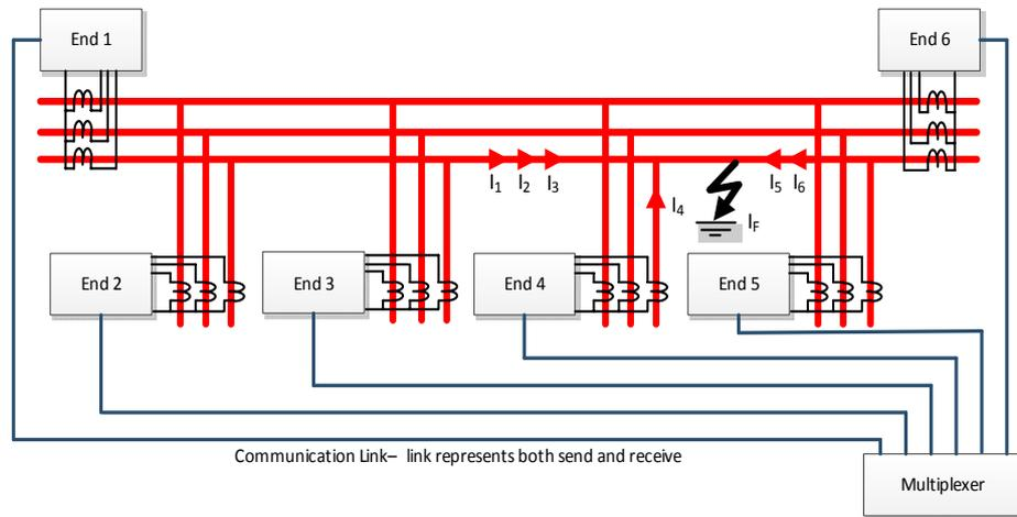
**Figure 1 - Multi-ended line differential protection principle**
