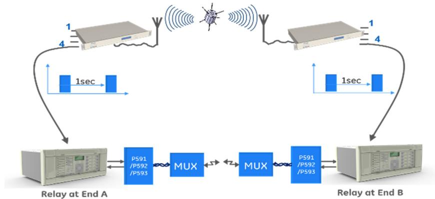
**Figure 2 - GPS-synchronized scheme**
