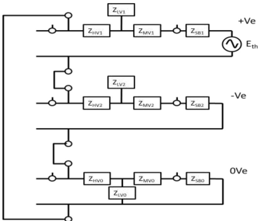
Figure 6-Sequence networks for the test case
