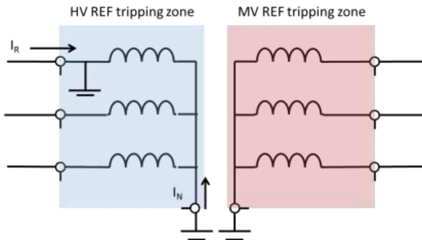
Figure 3-Current direction for a HV in-zone fault
