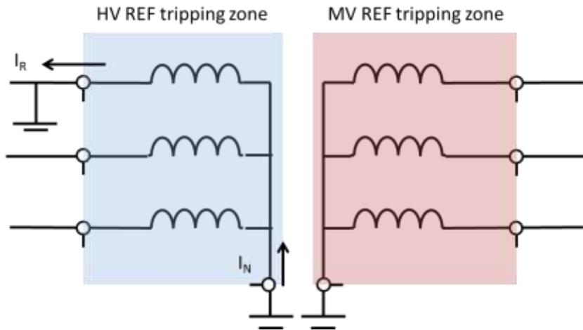
Figure 4- Current direction for a HV out of zone fault
