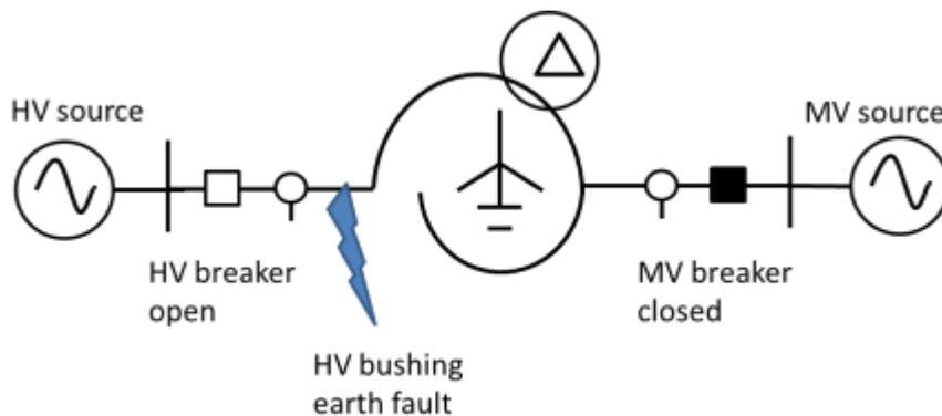
The network above was used to calculate the currents for a HV bushing fault. The following parameters were used. All impedances are in per unit on a 100 MVA base. All network resistances are ignored; hence all impedances are inductive reactances.
