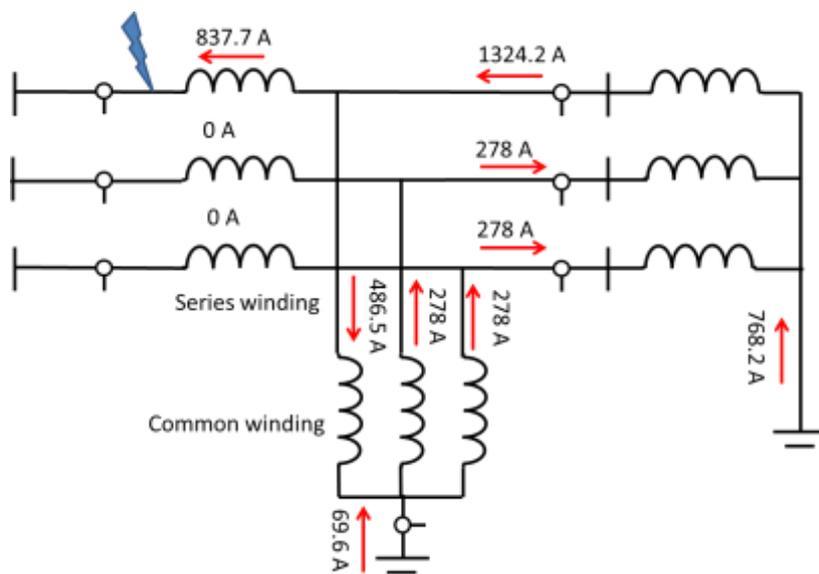
Figure 8- Current distribution for HV bushing earth fault with weak MV source
