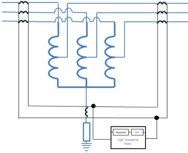
Figure 1-High Impedance REF CT connections
