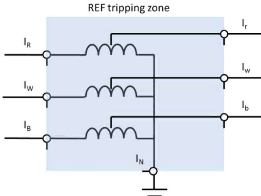
Figure 5-Low impedance REF applied to an auto-transformer
