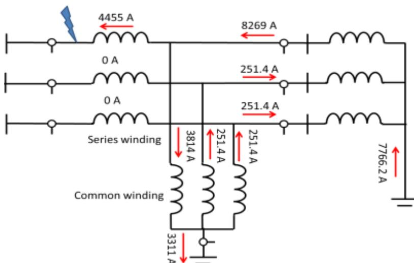
Figure 7-Current distribution for HV bushing earth fault with strong MV source
