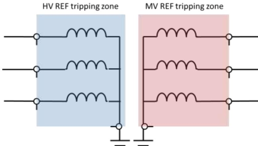
Figure 2-Low Impedance REF application when 2 earths are available
