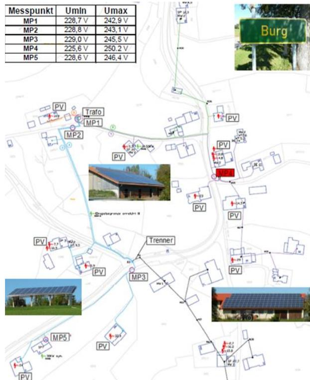
**FIGURE 3. Grid analysis via simulation**
