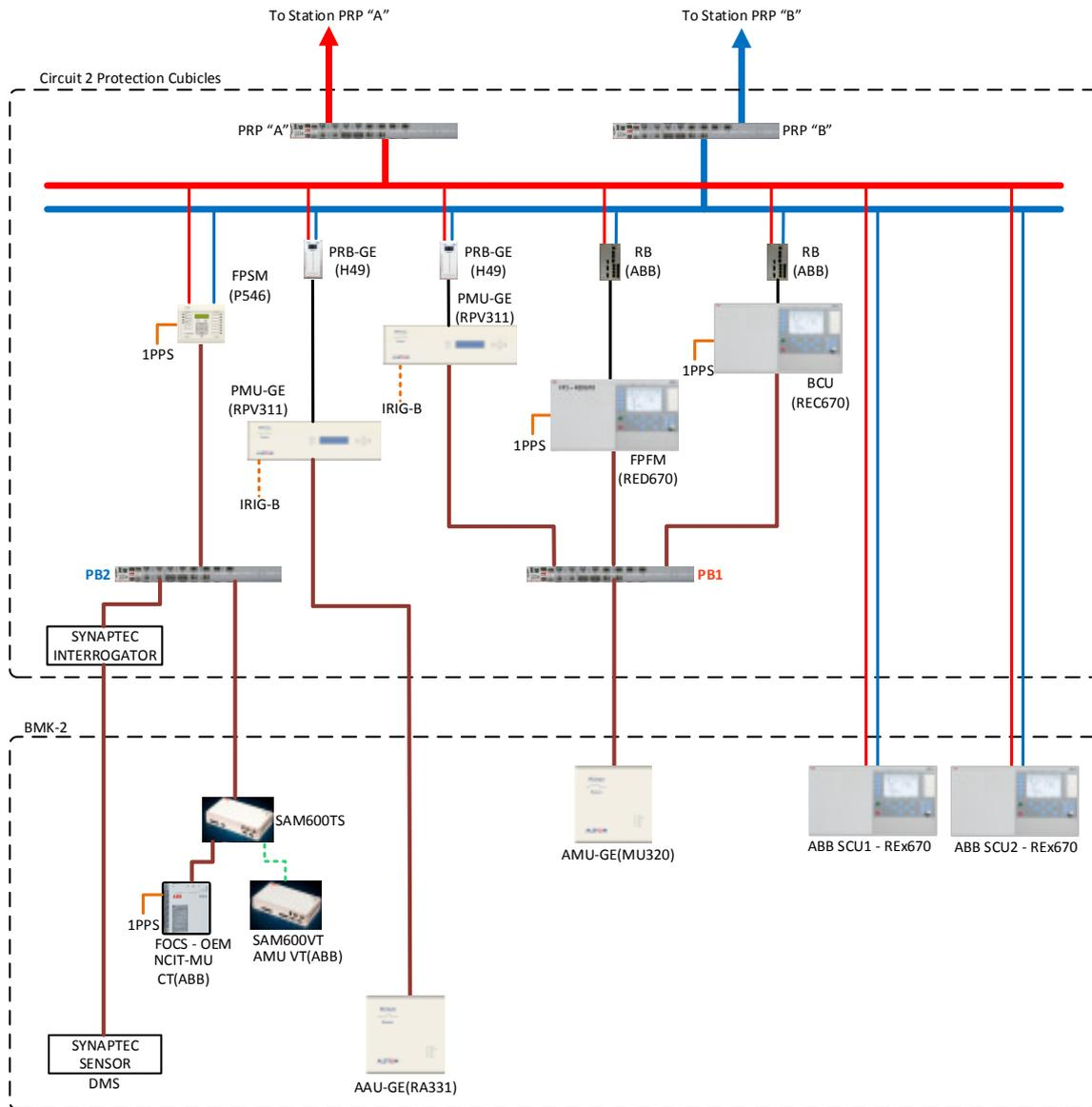
**Figure 5: Bay 2 system architecture at bay and process level**
