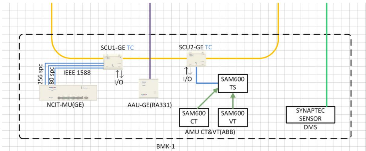
**Figure 4: Bay 1 system architecture at process level**
