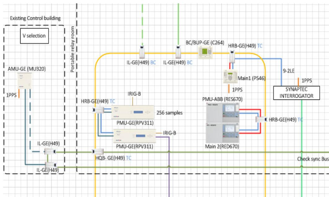
**Figure 3: Bay 1 system architecture at bay level**
