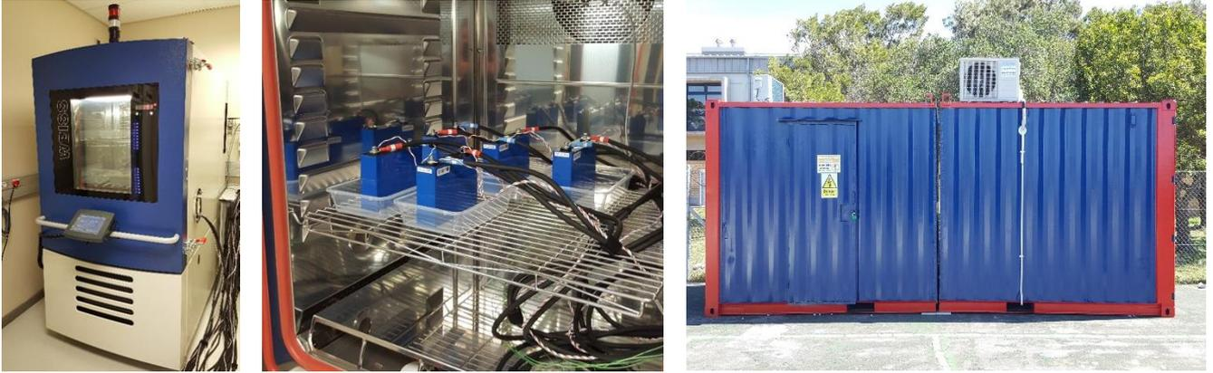
Fig. 3: Explosion proof temperature chamber for the testing of lithium-ion cells and air-conditioned container system for larger battery packs.
