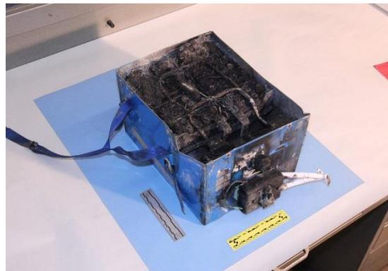
Fig. 2: Boeing 787 Dreamliner battery failure [3].
