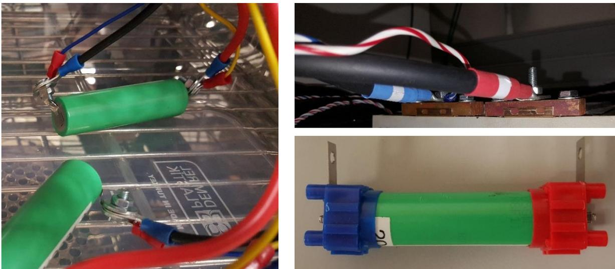
Fig. 5: Connectors used to allow for cells to connect to the battery testing equipment.
