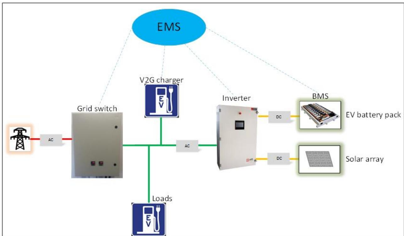
Fig. 2: The micro-grid layout of the pilot project. The EMS controls the energy flow from the inverter, V2G charger, grid and battery.
