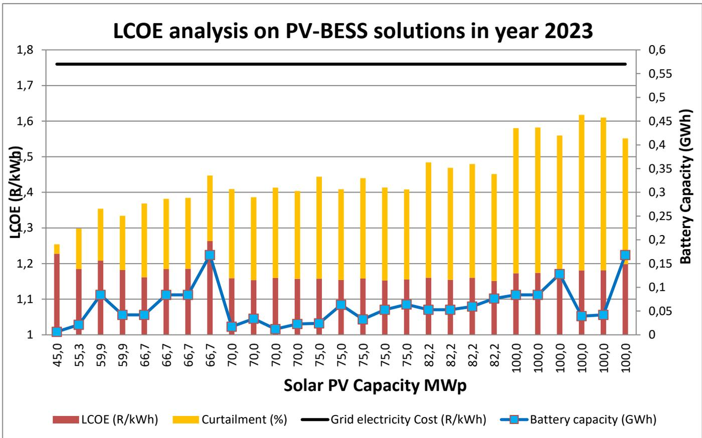
Figure 4 LCOE results on PV-BESS solutions with varying battery capacities and their respective % curtailments
