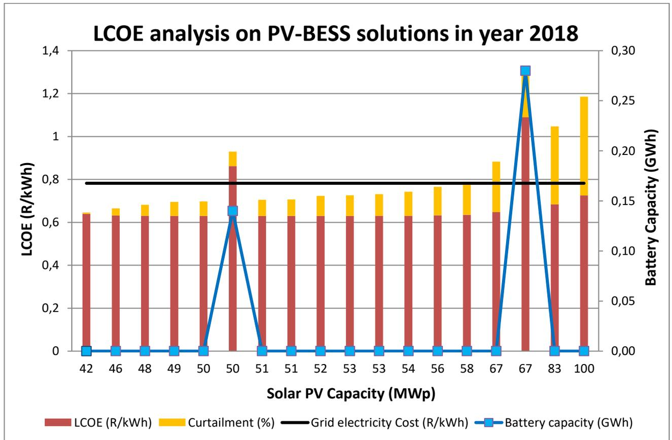
Figure 3: LCOE results on PV-BESS solutions with varying battery capacities and their respective % curtailment
