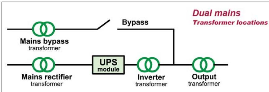
Fig. 8: Possible transformer locations for the dual mains configuration.
