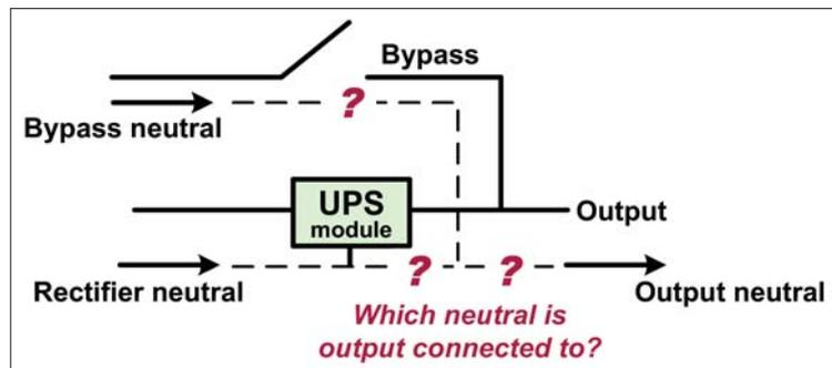
Fig. 4: How to create a single output neutral, with two input source neutrals.
