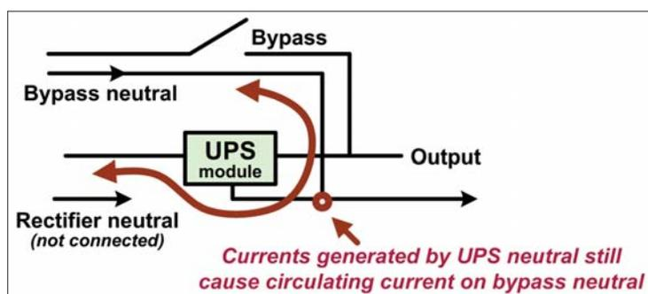
Fig. 6: Circulating current can still exist even if the rectifier input neutral is not connected.
