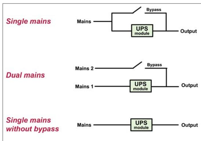
Fig. 1: Three basic configurations of mains and bypass for a UPS system.
