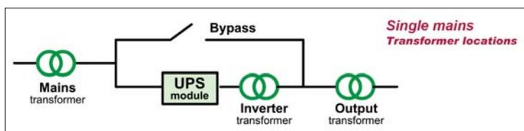
Fig. 7: Possible transformer locations in the "single mains" UPS configuration.
