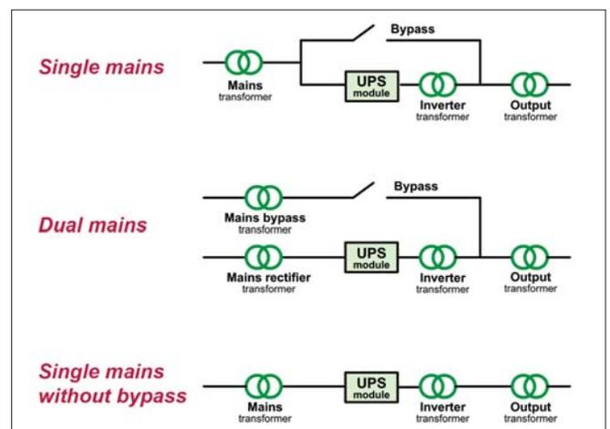
Fig. 2: Possible location of isolation transformers in the three basic UPS system configurations.
