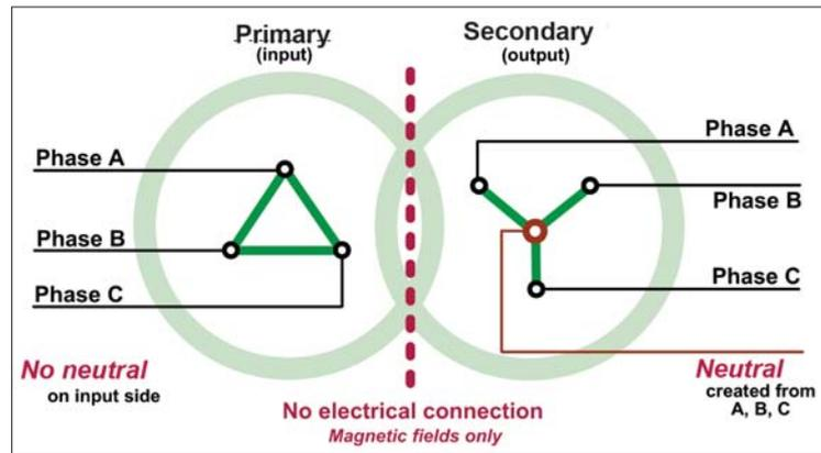
Fig. 3: Wiring diagram showing input and output connections to a power isolation ("deltawye") transformer.
