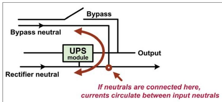
Fig. 5: Circulating current created by connecting two separate input neutral wires to create a single output neutral.
