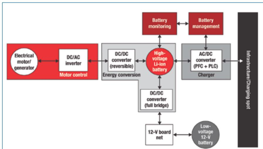
Fig. 1: System architecture of an electric vehicle.
