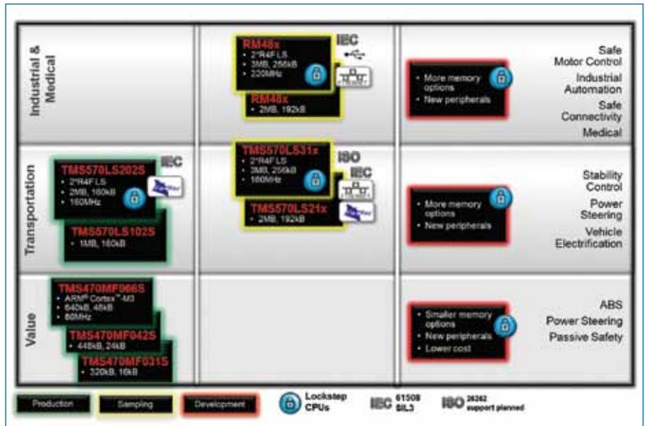
Fig. 3: Hercules safety microcontroller roadmap.
