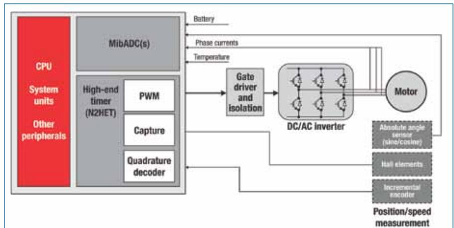
Fig. 2: Microcontrollers and power electronics for controlling the electric motor.
