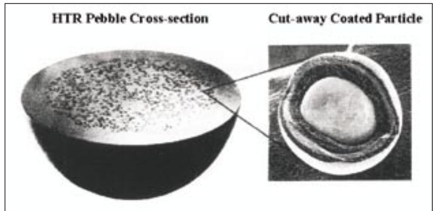
*'HTR Pebble cross-section' and 'cut-away coated particle'*
