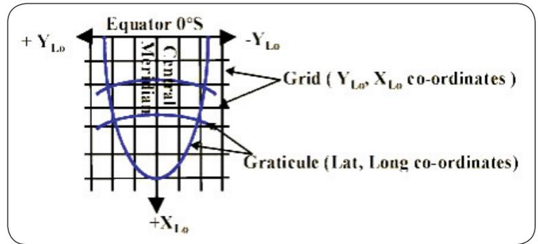
Fig. 8: The difference between the geographic coordinate system and the Mercator projection. (Credit: CD:SM)
