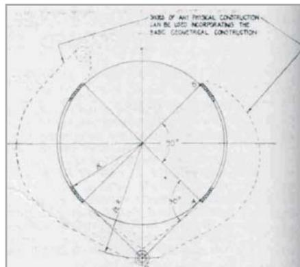
Fig. 1a: Geometrical construction of brake shoes.
