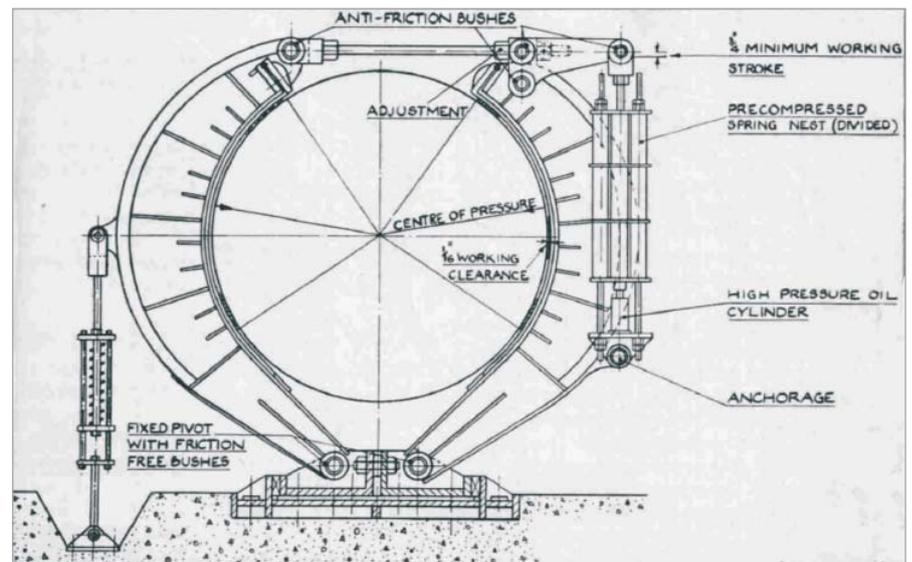
Fig. 2: Mechanical linkage between brake shoes and thruster.
