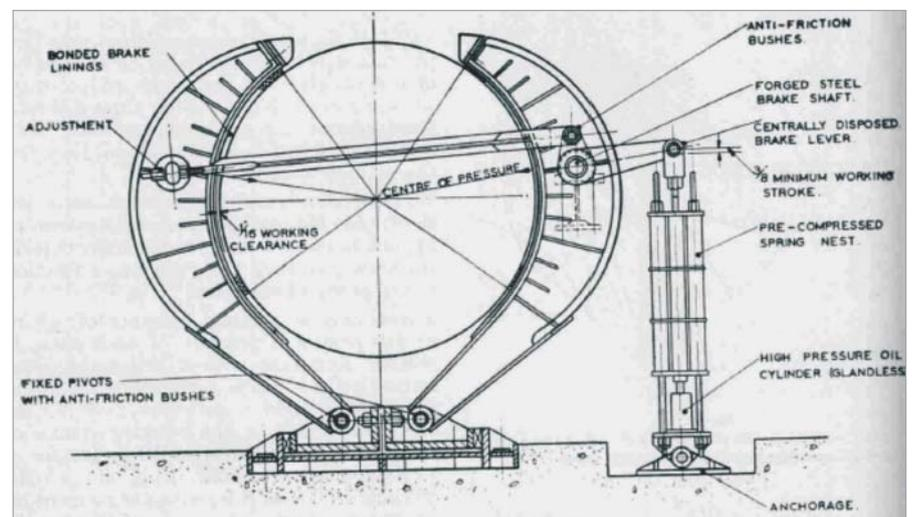
Fig. 3: Alternative arrangement of mechanical linkage.
