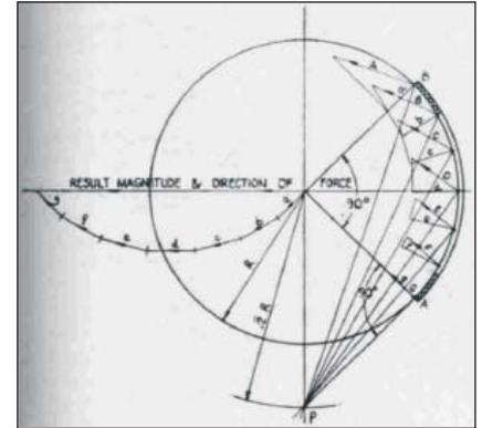
Fig. 1c: A.B.C – G – magnitude and direction of applied forces a.b.c – g – magnitude of resultant radial forces.
