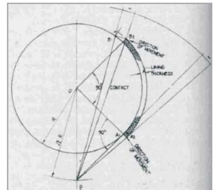
Fig. 1b: Analysis of movement of brake shoes.
