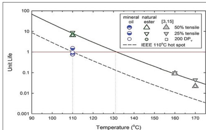
Fig. 3: Comparison of unit life of transformer for oil and natural ester [5].
