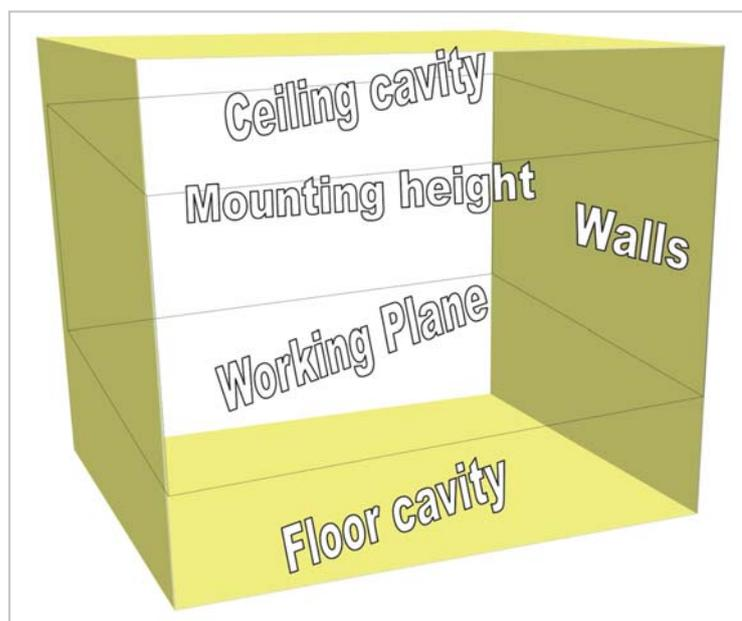
Fig. 1: Working plane and mounting heights.
