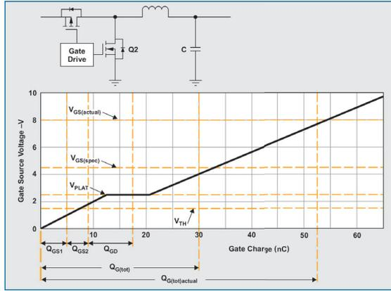
Fig. 10: Rectifier MOSFET gate driver and losses.
