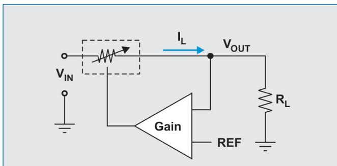
Fig. 1: Typical linear regulator.
