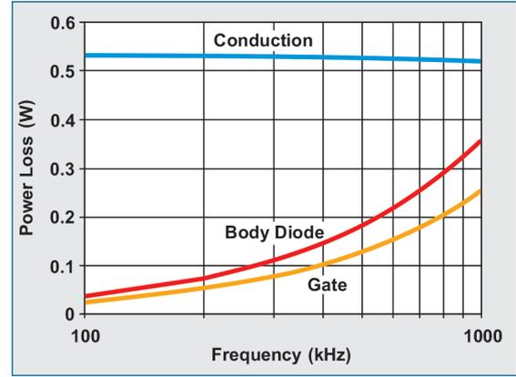
Fig. 11: Total rectifier MOSFET losses.
