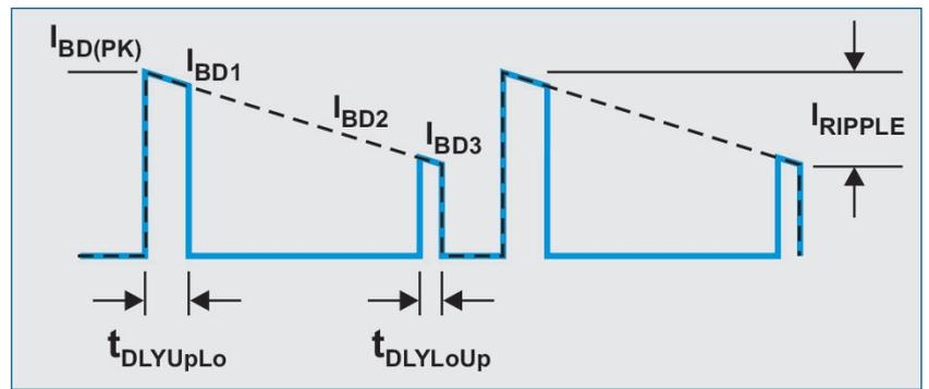
Fig. 9: Rectifier MOSFET body-diode current.
