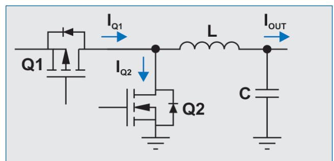
Fig. 4: MOSFET conduction losses.
