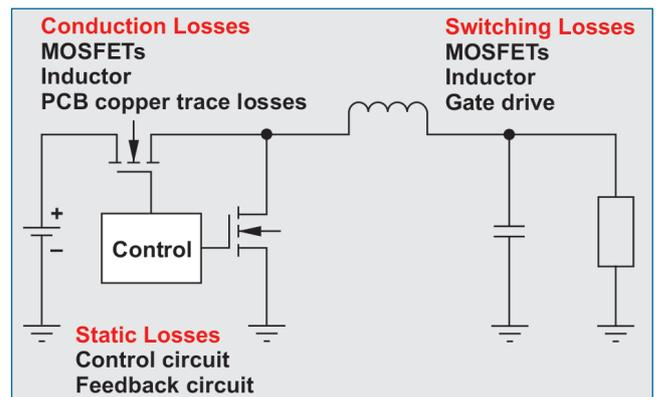
Fig. 3: Power-loss contributors in a buck switching regulator.
