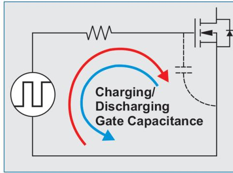
Fig. 6: Switch MOSFET gate losses.
