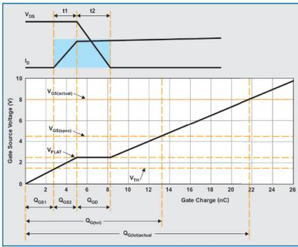
Fig. 5: MOSFET switching losses.
