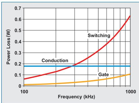
Fig. 8: Total switch MOSFET losses.
