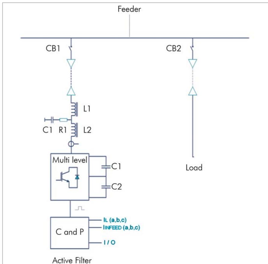
Fig. 1: Typical active harmonic configuration for industrial applications.
