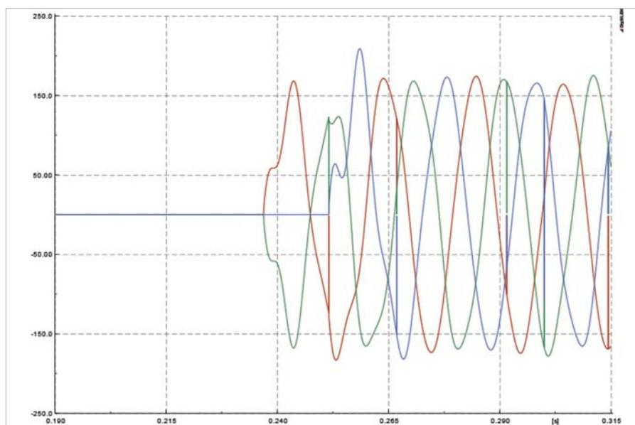
Fig. 6: Charged capacitor inrush current.
