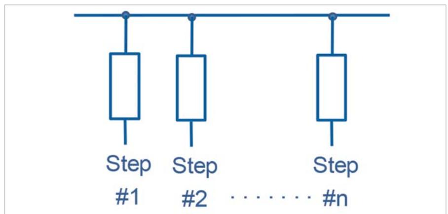
Fig. 3: TSC can be simplified as step controlled impedance.
