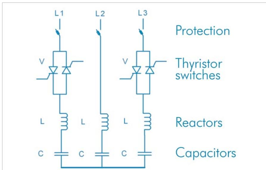
Fig. 4: Thyristor switched capacitor bank.
