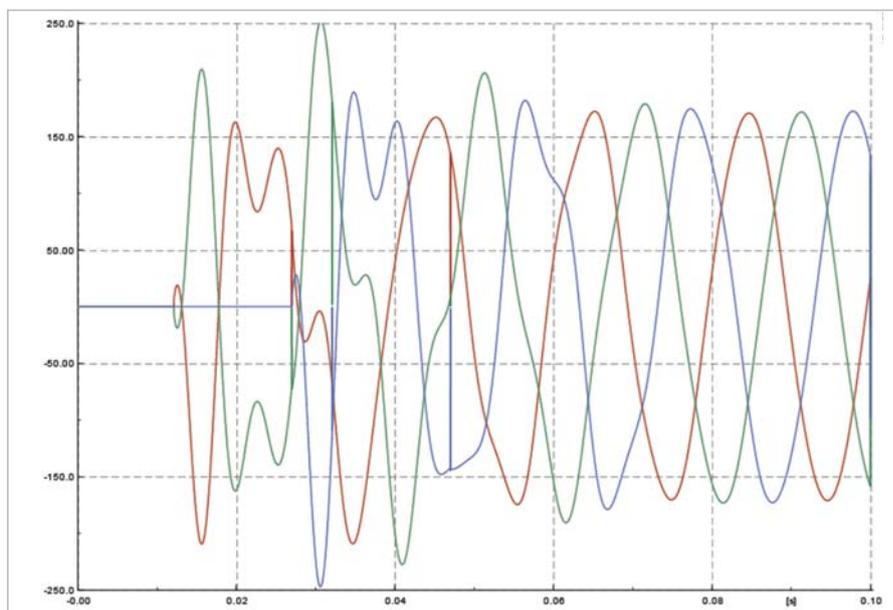
Fig. 5: Discharged capacitor inrush current.
