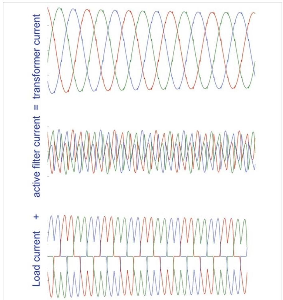
Fig. 2: Waveforms when all harmonics and fundamental reactive power is compensated.
