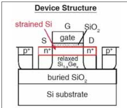
Fig. 4: Features of strained SOI MOSFET.
