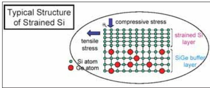
Fig. 3: Typical structure of strained Si.
