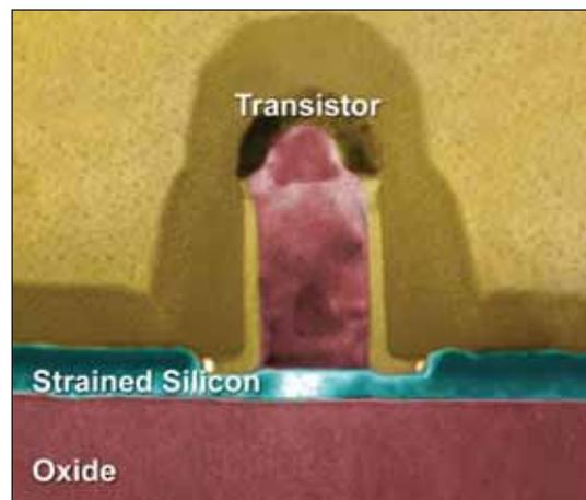
Fig. 6: IBM's strained silicon on insulator transistor.
