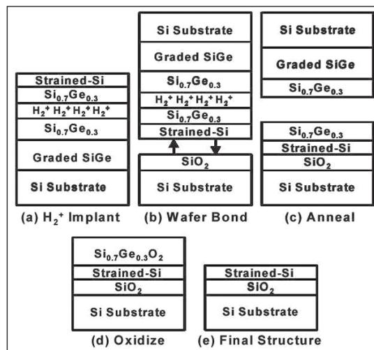
Fig. 1: SSOI fabrication process.
