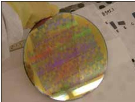
Fig. 5: AmberWave strained silicon wafer.
