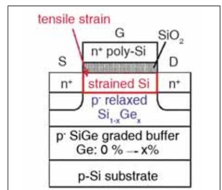
Fig. 2: Typical structure of strained-Si MOSFET.
